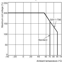
Note: The maximum coil voltage refers to the maximum value in a varying range of operating
